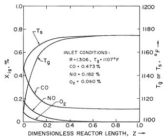
For the oxidizing gas mixture CO is completely used up, while in overall reducing atmosphere  $0_2$  is used up completely. As can be seen there is appreciable temperature gradient between the bulk and surface near the inlet, and both the temperature and composition profiles quickly develop to their final outlet values after the first 50% of monolith length.
